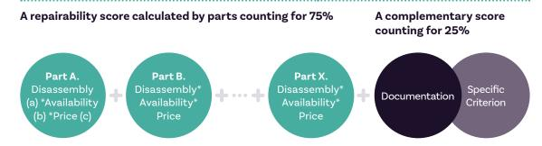
For each part : repairability of part A is calculated such as :  $R_A = \sqrt[3]{a * b * c}$
