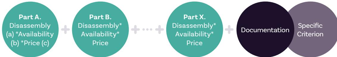
For each part : reparability of part A is calculated such as :  $R_A = \sqrt[3]{a * b * c}$
